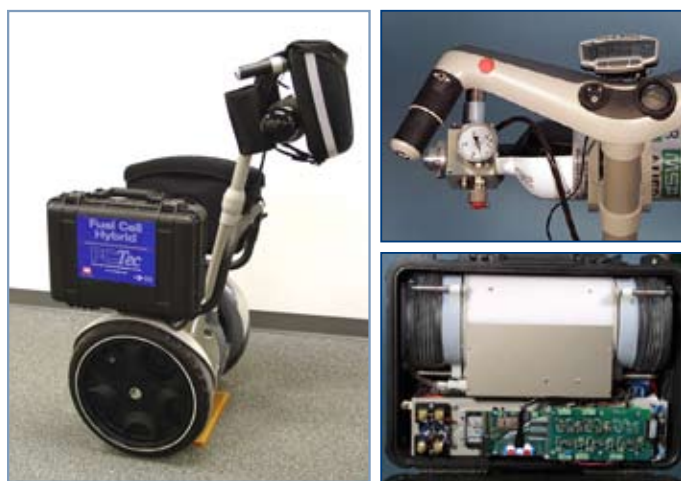
The FCTec integrated a 700-watt PEMFC into this first-of-its-kind battery powered Segway™ hybrid vehicle.
